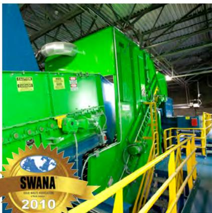
25 TONS-PER-HOUR SINGLE STREAM SYSTEM, APPLETON, WI
